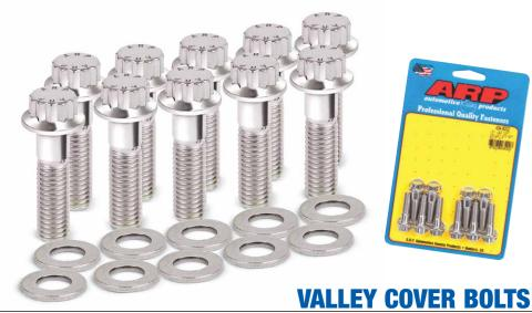
A companion to ARP's intake manifold bolts are these heavy-duty valley cover bolts, which come in black oxide finish 8740 or polished stainless steel with hex or 12-point heads. Nominally rated at 170,000 psi tensile strength.
